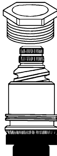
43066 AS-1R stem assy. 43067 AS-1L stem assy. 43068 AS-1R stem assy. with locknut 43069 AS-1L stem assy. with locknut
